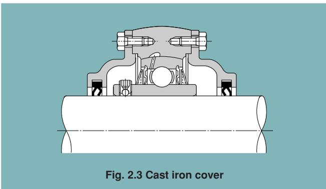
designed that when the shaft is inclined the rubber seal can move in the radial direction.
