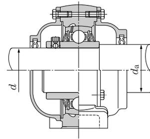
**Table 11.1 Bearing units with covers (for use with step shafts) and shaft diameters**
