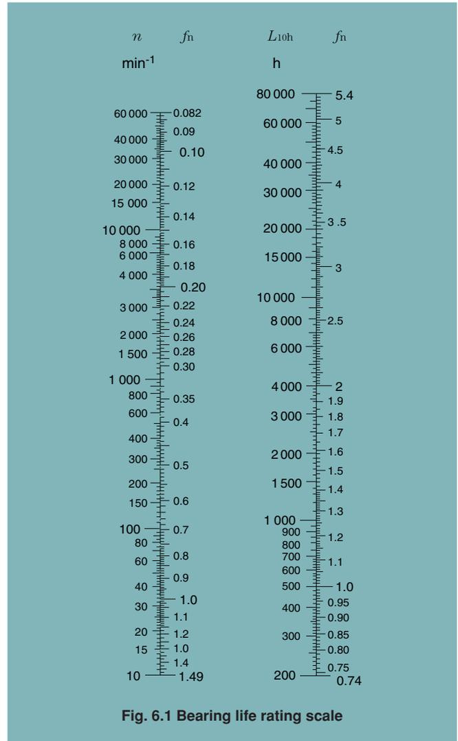
Fig. 6.1 Bearing life rating scale
