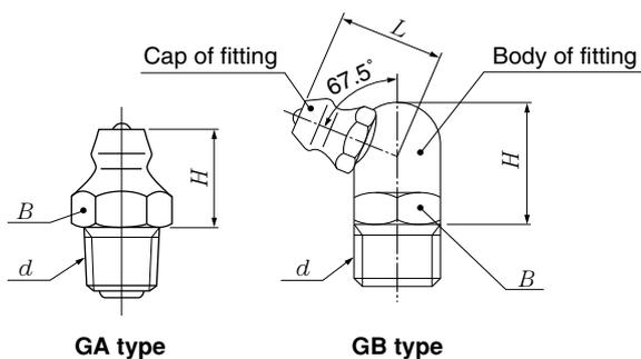
**Table 10.7 Grease fitting dimensions** GA type (Vertical type)
