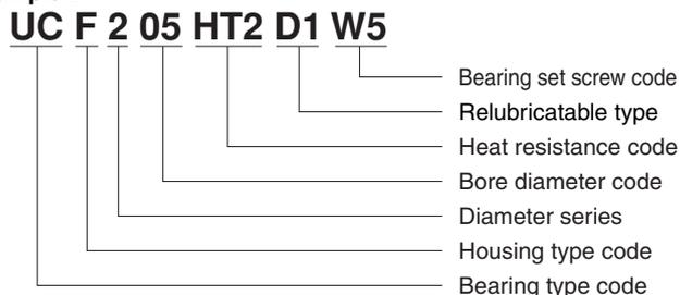
Bearing specifications for heat resistance and cold resistance are shown in Table 4.2.
