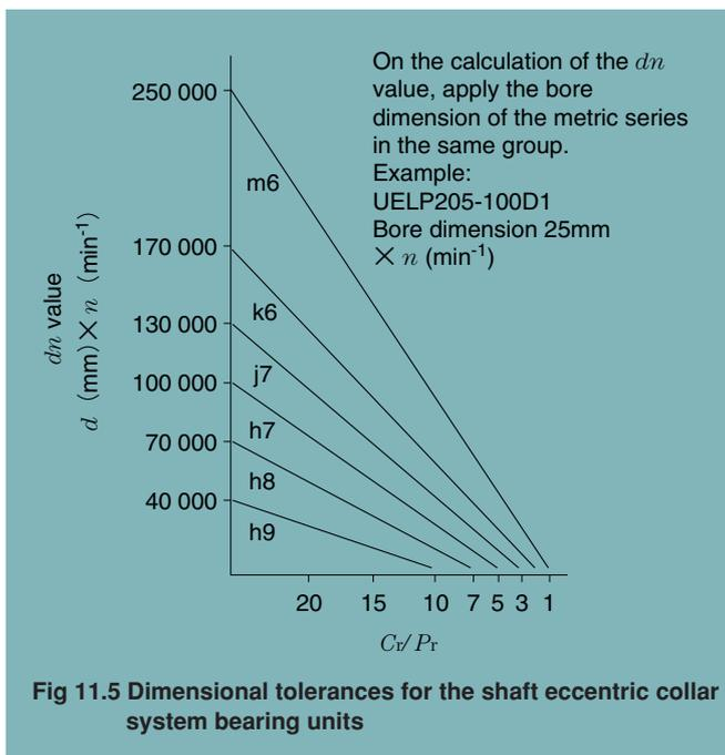
Fig 11.5 Dimensional tolerances for the shaft eccentric collar system bearing units
